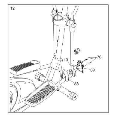
13. Have a second person hold the Handlebar (22) in place around the Upright (2).
