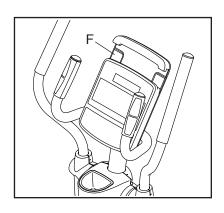
**secured in the tablet holder.** Reverse these actions to remove the tablet from the tablet holder.
