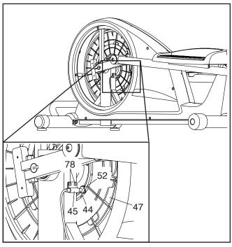
Next, rotate the Pulley (47) until a Magnet (52) is aligned with the Reed Switch (44). Slide the Reed Switch slightly toward or away from the Magnet. Then, retighten the M4 x 16mm Screws (78).
