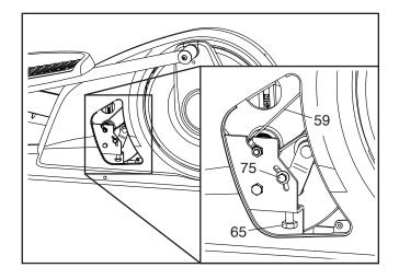
When the Drive Belt (59) is tight, tighten the Idler Screw (75). Then, reattach Access Cover (29) and plug in the power adapter.
